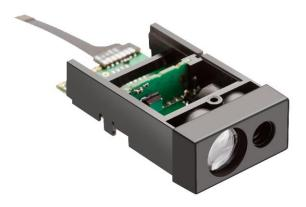
Egismos latest generation of Laser distance measurement modules offers measuring ranges up to 20 meters. The LDK Model 3 series are compact units with the smallest dimensions ever: only 48.9 x 26 x 13 mm. They are designed for users to easily connect the Laser measurement unit to a PC or an MCU through RS232 communication (UART TTL). The unit has a 1mm resolution and an accuracy of  $\pm$ 3.0mm along with a sampling rate up to 3 Hz.
